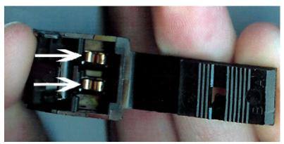
• Note the placement of the wire color. Pull the two wires out of the back of the connector. The terminal flange will be bent down near the terminal at this point.
